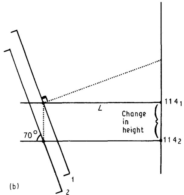
Figure 6 (a) Diagram illustrating the calibration geometry for a silicon calibration standard having  $[114]$  normal to the screen and the parameters  $\phi$ ,  $N$  and  $L$  in Equation 1. The pattern centre is  $[114]$ . (b) Diagram illustrating the height change part of the calibration routine. The distance between  $114_1$  and  $114_2$  is measured in screen coordinates.
