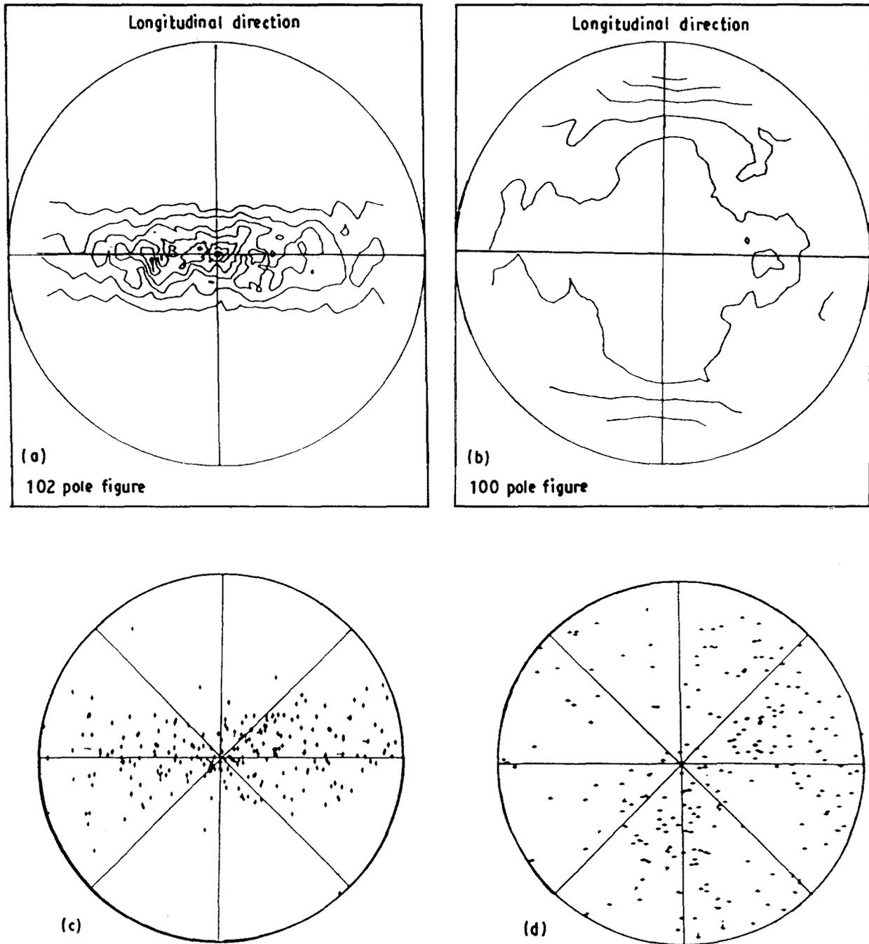
Figure 11 (a, b)  $[0001]$  and  $[10\bar{1}0]$  X-ray-generated pole figures, respectively, for zircaloy compared with EBSD generated pole figures for the same zone axes (c) and (d).
