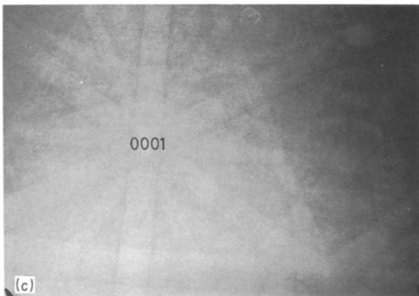
Figure 20 EBSD determined inverse pole figures from an aluminium alloy containing second-phase silicon particles. (a) Silicon particles which have recrystallized grains attached; (b) recrystallized aluminium grains. The two microtextures are complementary to each other. (Courtesy Jack *et al.* [82].) (c) EBSD from a hexagonal  $M_7C_3$ -type carbide which has lattice parameters  $a = 0.6921$  nm and  $c = 0.4508$  nm.
