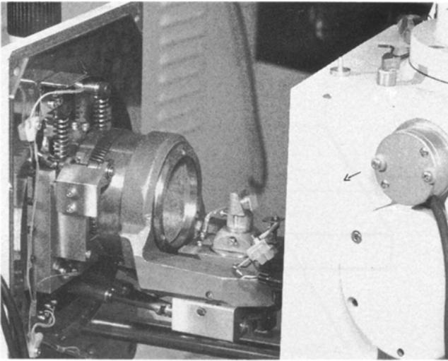
Figure 5 Photograph of a specimen mounted on its holder which is pre-inclined at 70.6° ready to be inserted into the microscope chamber.
