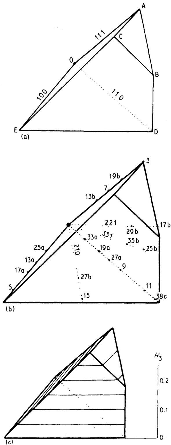
Figure 22 (a) One basic unit subvolume (1/48) of the fundamental zone. The locations of 100, 110 and 111 axes are shown. (b) Location of CSLs having  $\Sigma$  values up to 35 in the subvolume. CSLs misoriented on axes of the form  $uvv$  are omitted for clarity. (c) Sections in the  $R_3$  component of the  $R$ -vector through the subvolume parallel to its base. The  $R$ -vectors which lie in each section can then be shown in projection.
