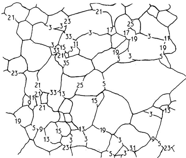
Figure 17 Mesotexture "map" showing the grain-boundary geometry of those grains in the micrograph in Fig. 1. CSLs are labelled with their  $\Sigma$  value and low-angle boundaries are labelled L. Unlabelled boundaries have non-special geometries.
