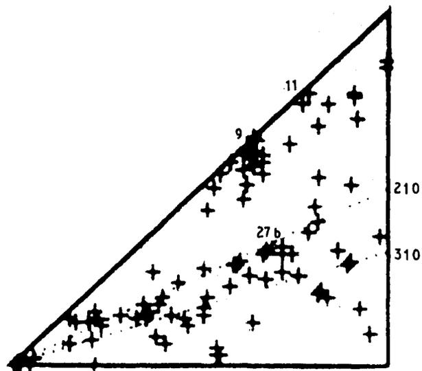
Figure 23 An example of an experimental mesotexture from an austenitic steel displayed in RF space. A projection having  $R_3 < 0.05$  showing clusters of low-angle boundaries and  $\Sigma = 9, 11$  and  $27b$  CSLs.
