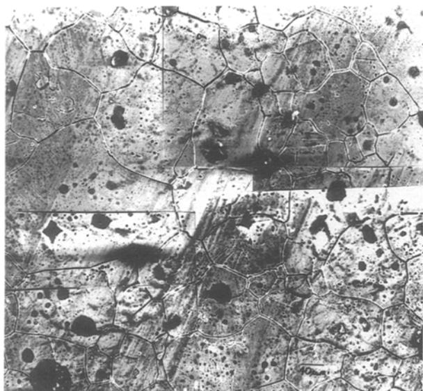
*Figure 1* Scanning electron micrograph of annealed nickel. The microtexture of every grain has been measured using EBSD. This information is displayed in Fig. 24 (see Section 7), and the accompanying "mesotexture map" is shown in Fig. 17 (see Section 5).
