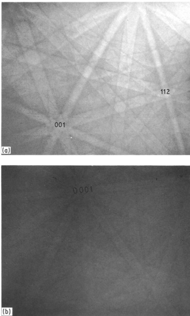
Figure 7 EBSD patterns from (a) a face-centred cubic material (nickel), and (b) a close-packed hexagonal material, Zircaloy. Some major zone axes are marked.
