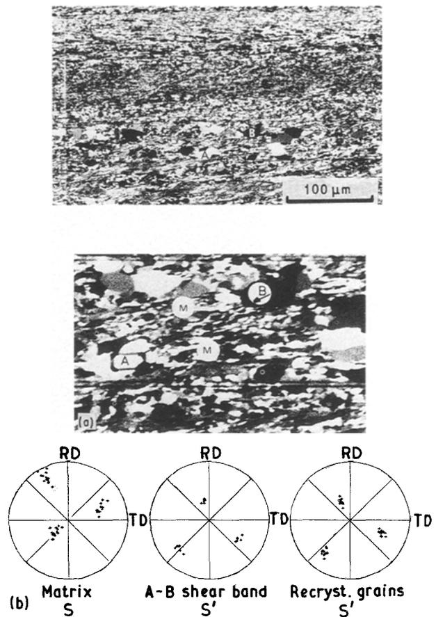
Figure 14 Recrystallized grains having an S-type texture nucleating in shear bands in deformed aluminium. (a) Micrograph showing newly recrystallized grains; (b) EBSD-determined pole figures from the new grains in (a). Courtesy Hjelen and Nes [48].
