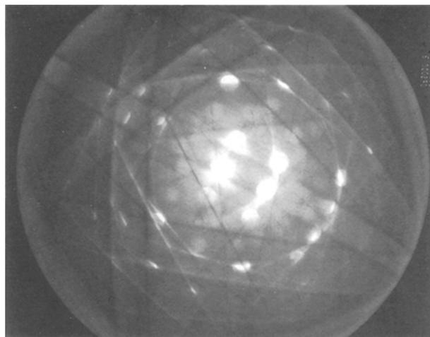
*Figure 2* Convergent-beam diffraction (CBED) pattern from an austenitic steel. The beam direction is close to 113.
