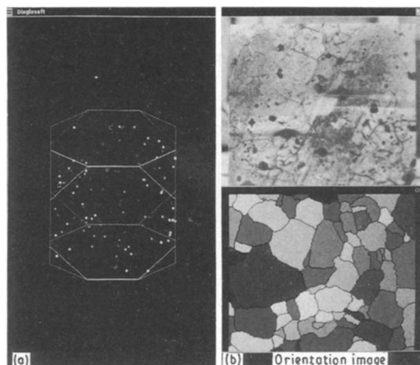
Figure 24 (a) "Orientation image" of the portion of nickel polycrystal shown in Fig. 1. The grains are colour coded according to their orientation as shown in (b) recorded in RF space.
