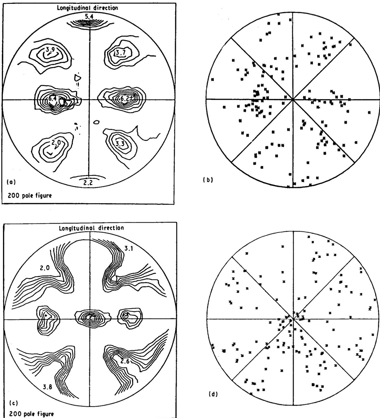
Figure 10 Pole figures from an Al-Li alloy rolled to sheet. (b) and (d) are EBSD-determined microtexture subsets (50 grains each) of the X-ray-determined pole figures in (a) and (c), respectively. (a) and (b) show the recrystallized texture from the sheet edge and (b) and (d) show retained rolling texture from the sheet centre. There is a good match between (a) and (b), and (c) and (d), respectively.
