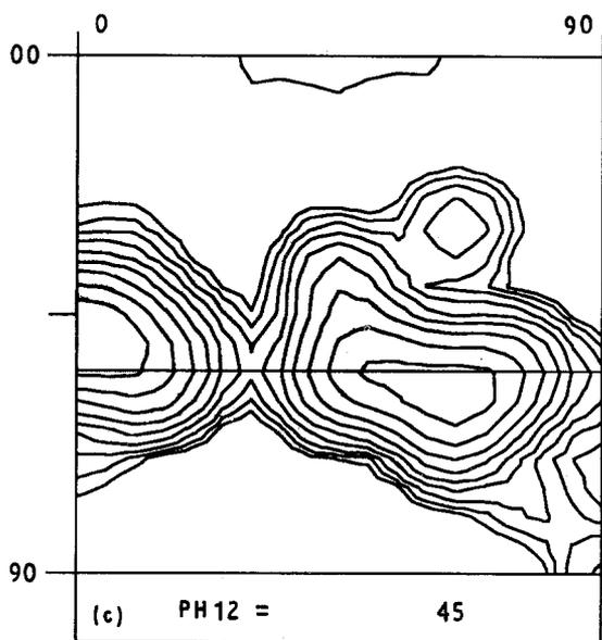
Figure 12  $\phi_2 = 45^\circ$  sections of ODFs from a rolled and annealed steel sheet. (a) X-ray-generated macrotexture; (b, c) EBSD generated microtextures from (b) of only the smallest grains, and (c) all other grain sizes in a 160 grain sample population [37]. (Courtesy of P. Van Houtte.)
