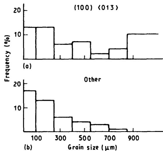
Figure 15 EBSD-determined microtexture of an Al-SiC composite shown as frequency histograms of grain sizes of grains having microtexture (a) close to  $\{100\}\langle 013 \rangle$ , and (b) all other microtextures. (Courtesy Juul Jensen *et al.* [50].)
