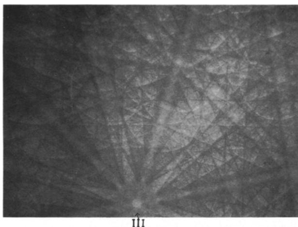
Figure 4 Electron back-scatter diffraction (EBSD) pattern from a broken tungsten filament. Note the wide angular range compared with the CBED or SAC pattern. The crystal structure is body-centred cubic. Some major zone axes are marked.
